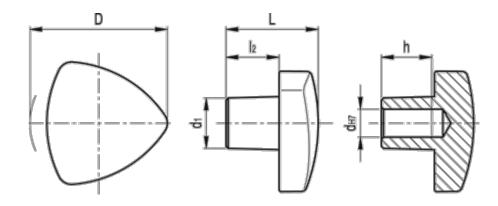
$\begin{array}{lll} D & = 32 \\ d1 & = 12 \\ d \ H7 & = 6 \\ h & = 12 \\ L & = 21 \\ l2 & = 12 \\ Weight (g) = 58 \end{array}$
